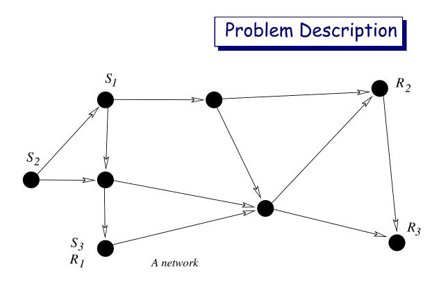
Vertices: V Edges:  $E \subseteq V \times V$ ,  $e = (v, u) \in E$ Edge capacity: C(e)(=1)Network:  $\mathcal{G} = (V, E)$ Source nodes:  $\{v_1, v_2, \dots, v_N\} \subseteq V$ Sink nodes:  $\{u_1, u_2, \dots, u_K\} \subseteq V$   $\mu$  (rate one) input random processes at v:  $\mathscr{X}(v) = \{X(v, 1), X(v, 2), \dots, X(v, \mu(v))\}$
