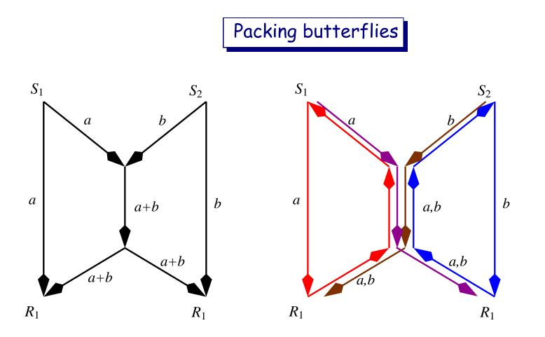
Generalizing the flow decomposition of butterfly networks we can formulate a linear program to solve Class II network coding problems!
