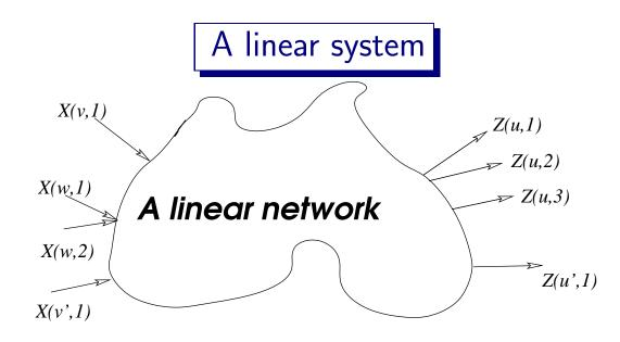
Input vector:  $\underline{x}^T = (X(v, 1), X(v, 2), \dots, X(v', \mu(v')))$
